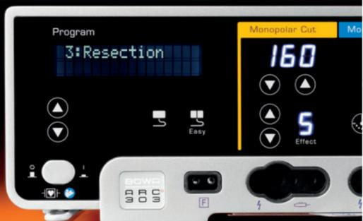
The resection program allows for the use of 300 W for vaporisation with monopolar resectoscopes
